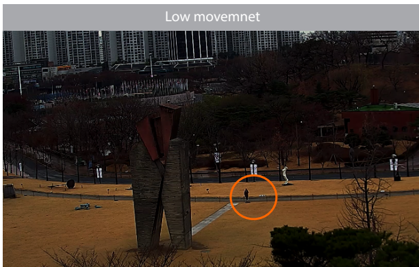
WiseStream II OFF : 7162kbps WiseStream II ON : 1685kbps
